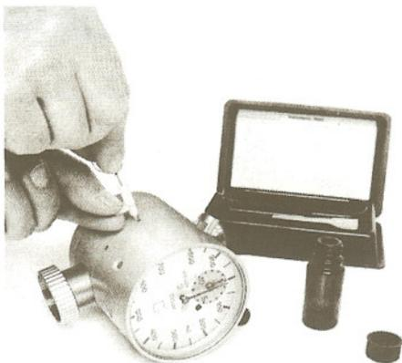
Fig. 11 Lubrication of the bearings
