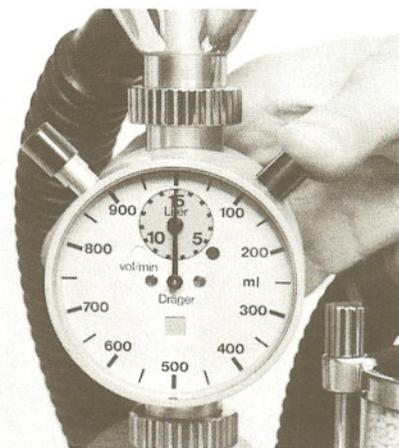
Fig. 4 Release of indicator hand for tidal volume
