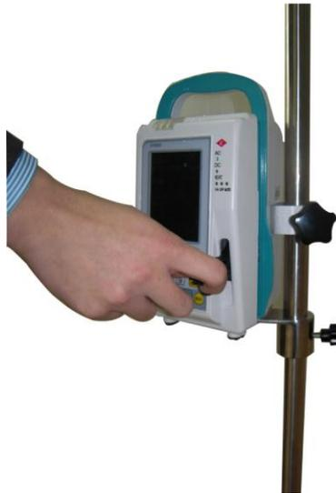
Fig 6-1 pull the door switch
