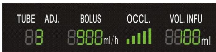
There are IV sets options: tubing types options, adjustment options, BOLUS rate options, occlusion detector sensitivity level options from left to right in turns. When the parameters are selected, the black frame of these parameters will be blinking. In addition, on the right of this area, there is accumulated infusion volume display value area
