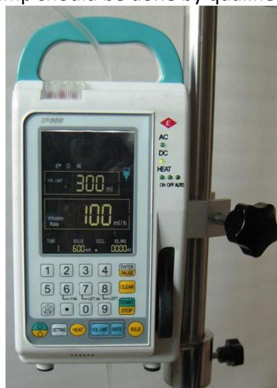
Fig 1-1 IP300 infusion pump appearance
