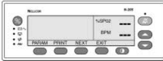
**Figure 4-1: Service Function Softkeys**
