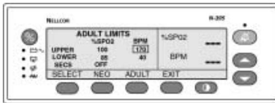
Figure 3-6: Adjusting High Pulse Rate Alarm
