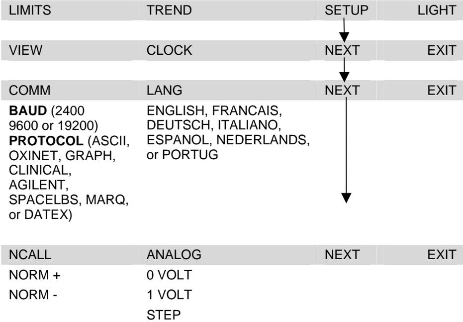
Press the Softkey under the desired parameter then press EXIT to return to the user menu.
