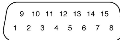
**Figure 10-3: Data Port Pin Layout**
