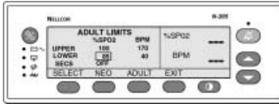
Figure 3-5: Adjusting % SpO2 Lower Alarm Limit
