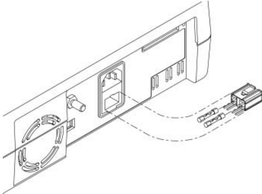
**Figure 6-1: Fuse Removal**
