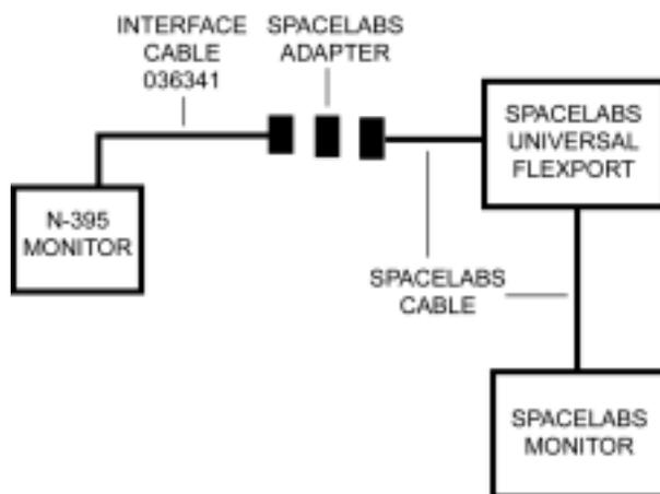
**Figure 10-2: SpaceLabs Connection**
