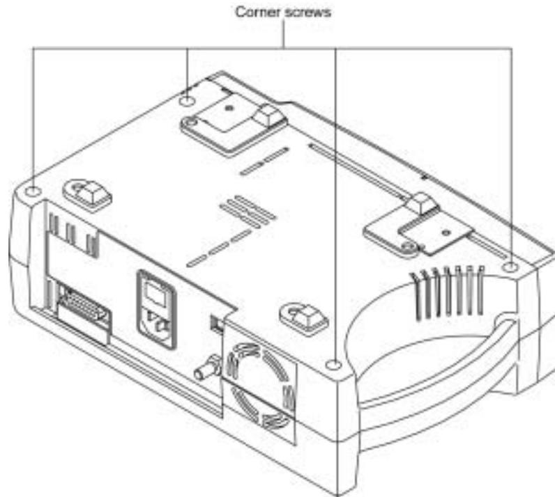
**Figure 6-2: N-395 Corner Screws**
