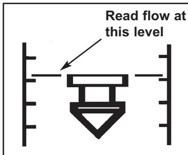
Each flow control valve is positioned directly underneath the flow tube assembly to which it corresponds, and the control knob is colour-coded for the gas which it controls.
