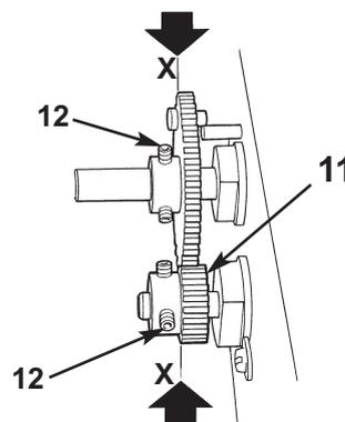
23. Tighten the grubscrews (12) to secure the N<sub>2</sub>O gear.
