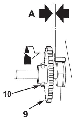
21. Distance the inner face of the O<sub>2</sub> gear (9) with a 0.1 mm feeler gauge at 'A'.
