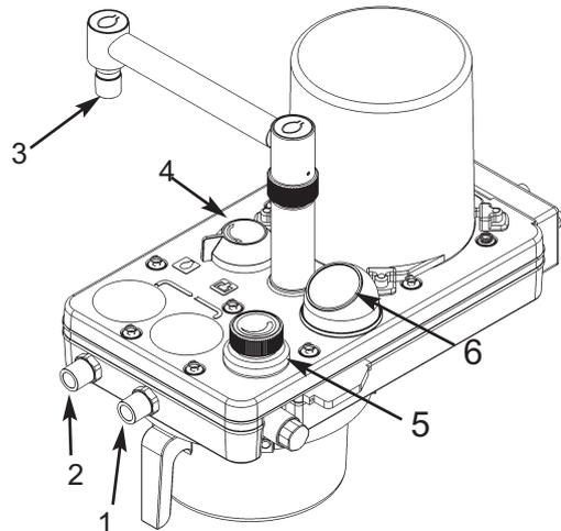
4. Release the oxygen flush valve. Check that the pressure is maintained in the system with less than 200 ml/min fresh gas delivered into the breathing system, showing that no leaks are present.
