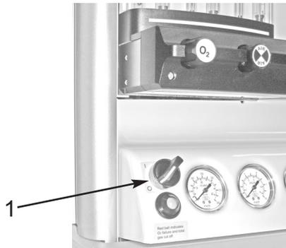
The Gas Delivery Switch (1) operates on the oxygen supply and must be in the 'On' position for normal operation of the anaesthetic machine.
