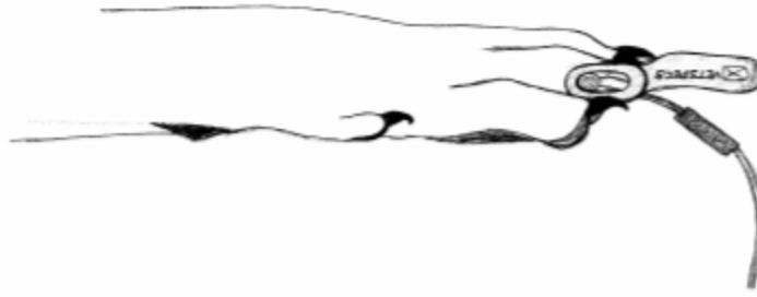
Sketch 6: The leg/toe sensor on a toe of dogs.
