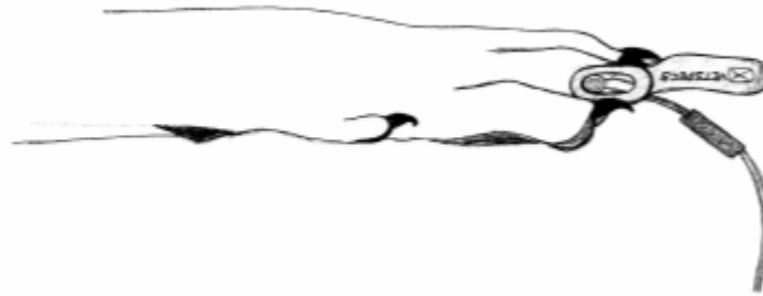
Sketch 4: The leg/toe sensor on a toe of dogs.
